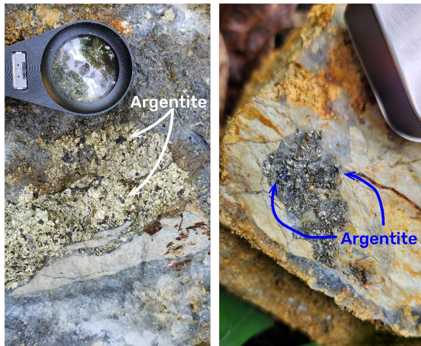
Figure 3. Photos of hand specimens from the El 20 historic workings showing pyrite-rich clusters with coarse-grained argentite (black spots).
