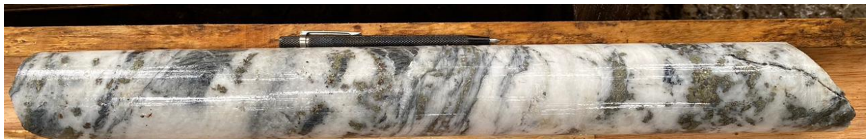
Figure 4. Hole SAAGDH373, sample 7921 from 188.62 to 189.29 metres in depth, returning 7.35 g/t Au and 1,258 g/t Ag in a massive quartz vein with clusters of sulfides, mainly pyrite and argentite (silver sulfide).
