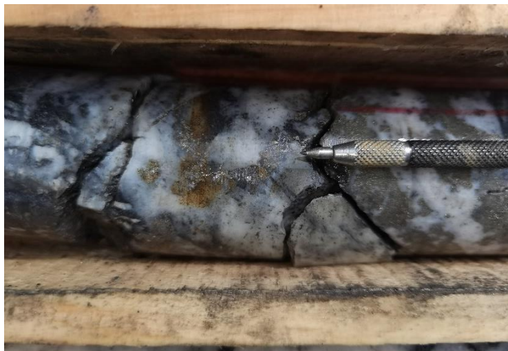
Figure 2. Core photo from hole DH279 at 183.85 m depth in Los Naranjos shoot with silver sulfosalts and sulfides.
