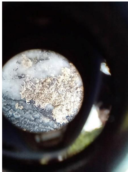
Figure 2. Abundant coarse (up to 2 cm x 1.5 cm) electrum in hole DH276. Coarse electrum correlates with high-grade assays.
