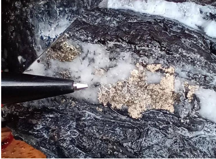
Figure 4: Abundant coarse (up to 2 cm x 1.5 cm) electrum in deeper Naranjos drill holes pending assay. This is some of the coarsest and more abundant electrum observed in core to date. Coarse electrum generally correlates with high-grade assays.
