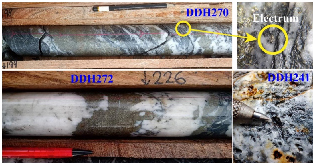
Figure 2. Drill core pictures showing common styles of mineralization within the Naranjos vein. Hole DH270 shows plus millimetre-scale electrum, and hole DH241 shows fine wire silver.
